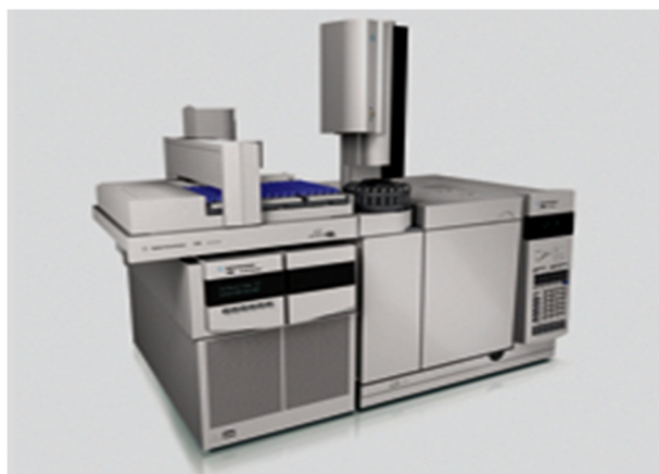
Figura 18. GC-MS/MS (QqQ) Agilent Technologies
