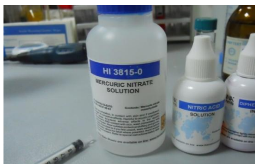
Figura 7. Kit de determinare a clorurilor HI 3815 (Hanna Instruments)
