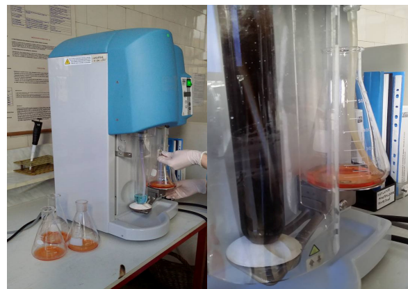
Dosing of ammonia
